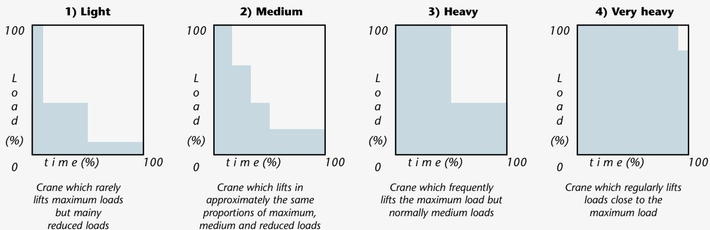
Check, on the basis of the state of stress intended for the crane, that the limits of use, type of service and n° of cycles intended in 10 years of work is not in contrast with the following table.
