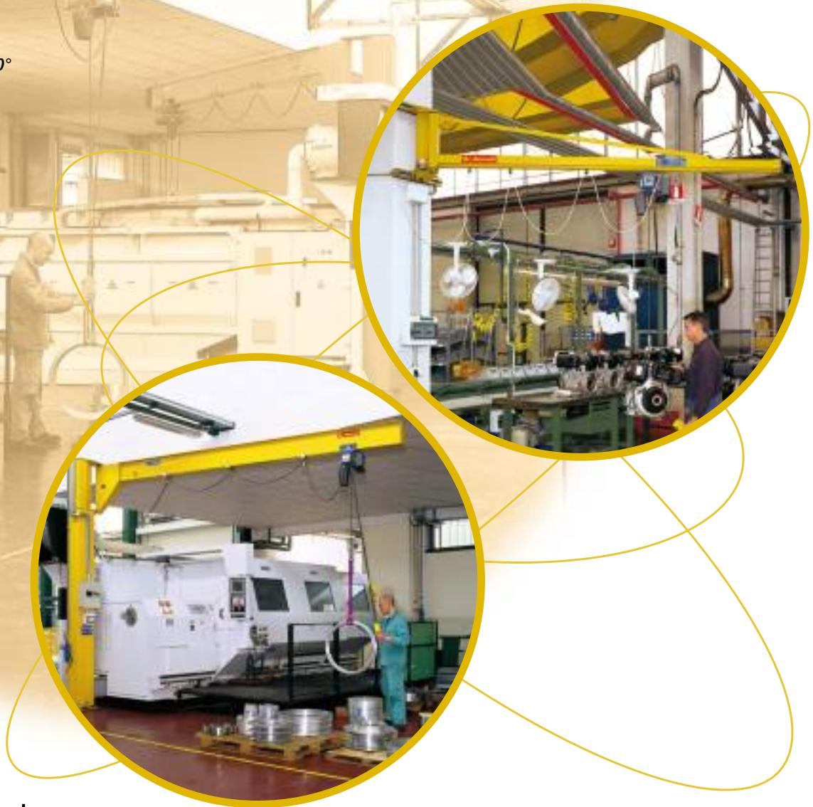
The manually rotated **jib cranes** in the **GBA"column" series** and the **GBP "wall" series** are designed for the handling of goods inside a plant, in a square or to serve operative positions.
