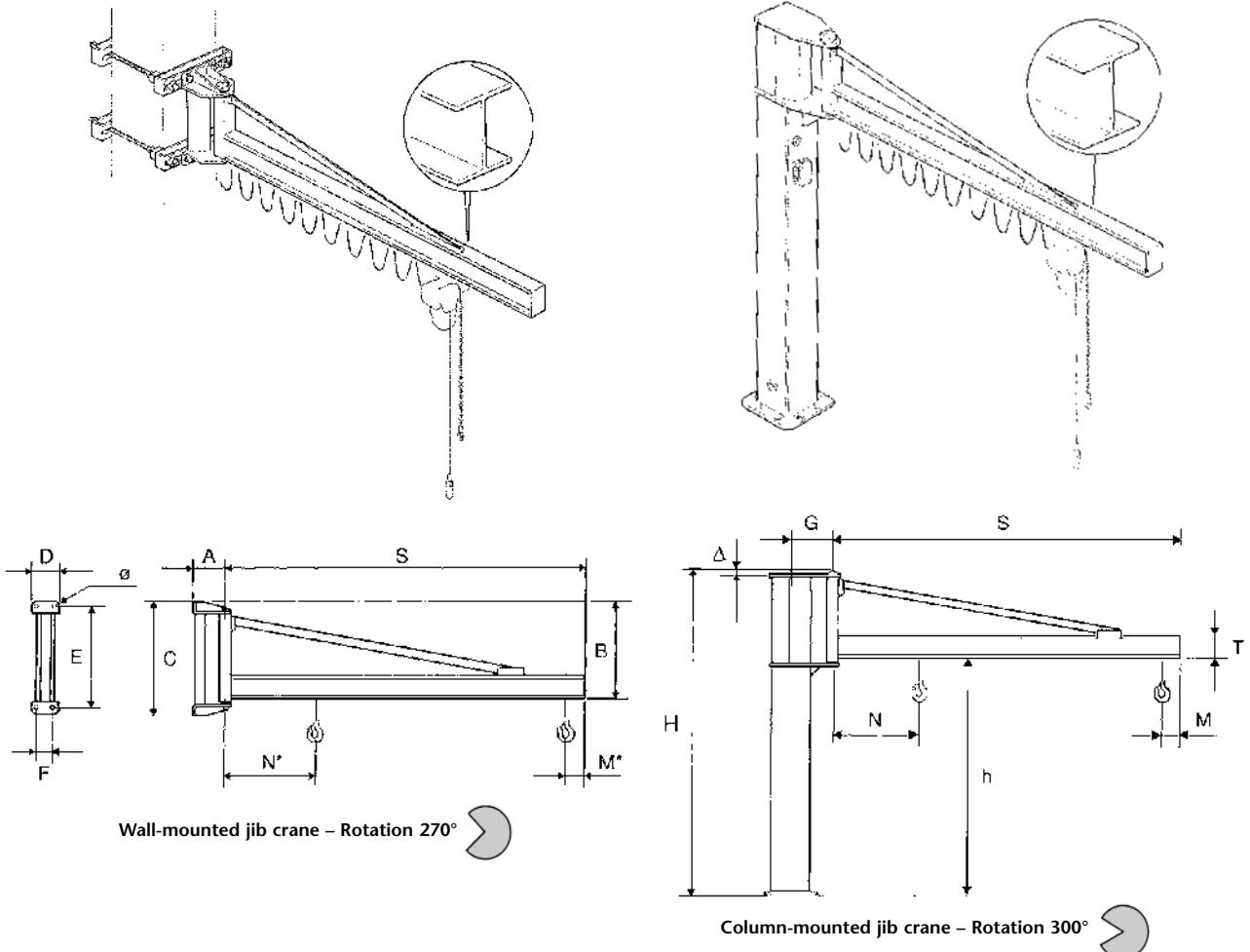
Heights M\* and N\* for wall-mounted jib cranes: see corresponding heights relative to column-mounted jib cranes
