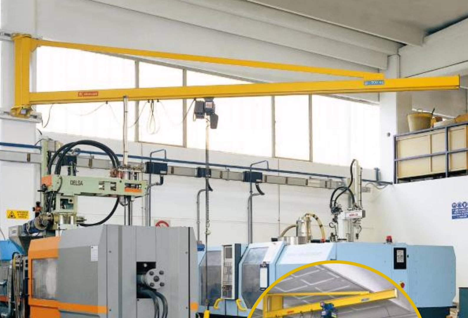
available space at a height due to the absence of staybolts and allows the maximum use of the hook run. The arm allows the addition of electrical or mechanical push-trolleys.
