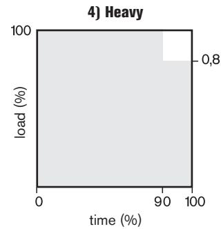
Hoists which regularly lift loads approximately equal to the maximum load.
