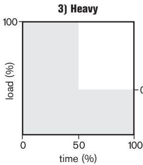
Hoists which frequently lift the maximum load but normally medium loads.
